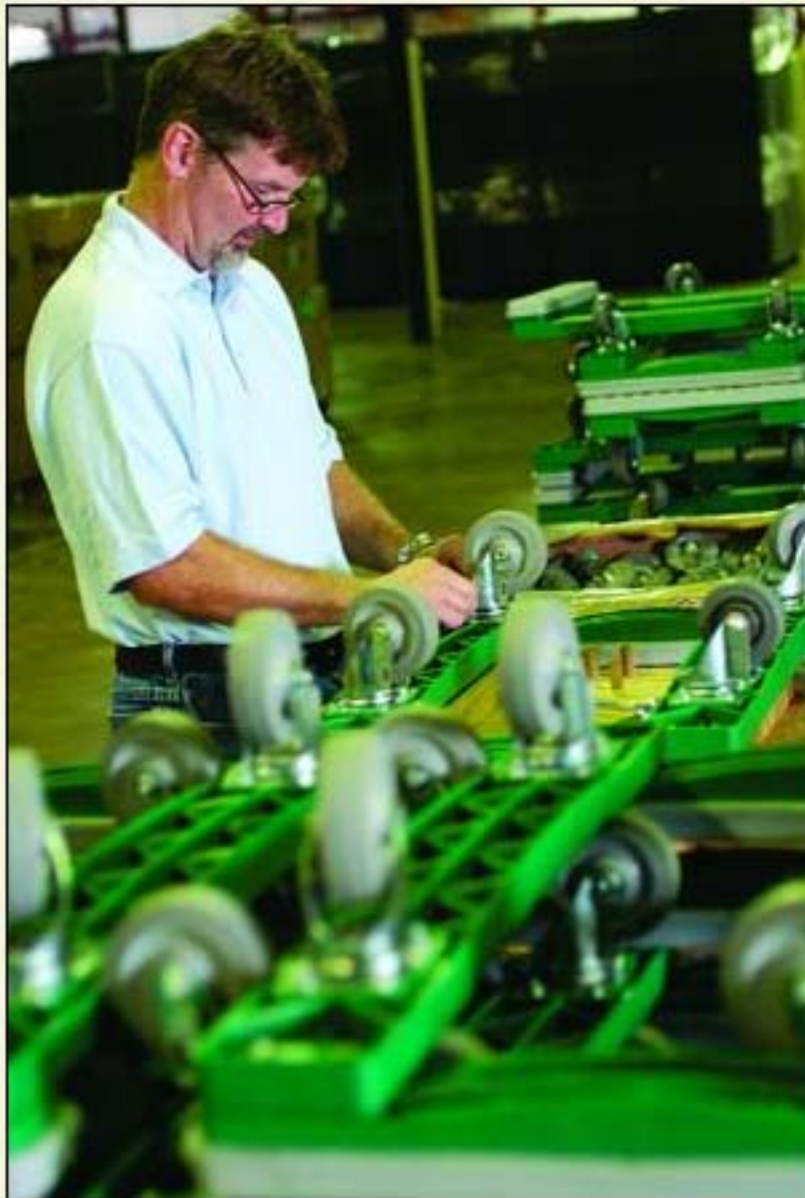
GEORGE WOLBER, research and development guru for Associated Plastics in Ada, attaches wheels onto plastic, recyclable dollies that are manufactured at the plant. The plastic dollies are competing with traditional furniture dollies of plywood, 90 percent of which are made in China or in other Asian countries. (Photo by Randy Roberts)
